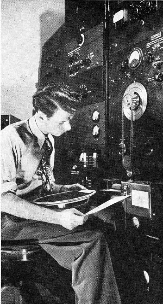
TWO SIDES OF A WALL —When a Receiver Division engineer becomes suspicious of a loudspeaker, he can bring it to this lab and run off a complete response curve in a few minutes. The loudspeaker is mounted in an opening in a wall between the
