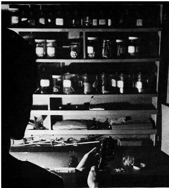
SWITCHES TO ORDER —Instead of ordering specially made samples of complicated wafer switches and waiting weeks for shipment, engineers in one Receiver lab assemble their own at this cabinet, which contains all necessary parts
