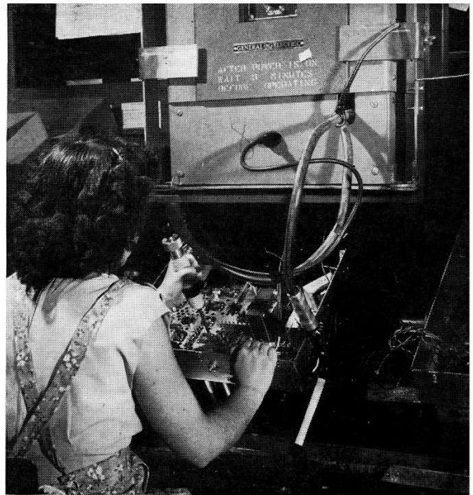
WELDING REPLACES SOLDERING —With electronically controlled resistance welding, this operator is able to weld 15 grounding ribbons and one resistor lead to the chassis of a television set during the two-minute time cycle. A snap-action switch built into the welding electrode applies current automatically
