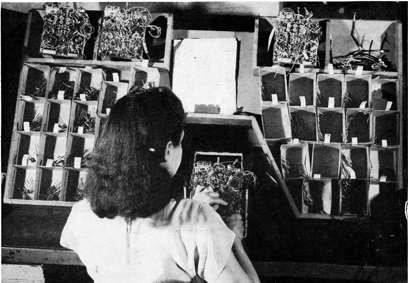
ORGAN-TYPE CONSOLE —For small production runs in Transmitter Building, long time cycles are most economical. Here one operator
